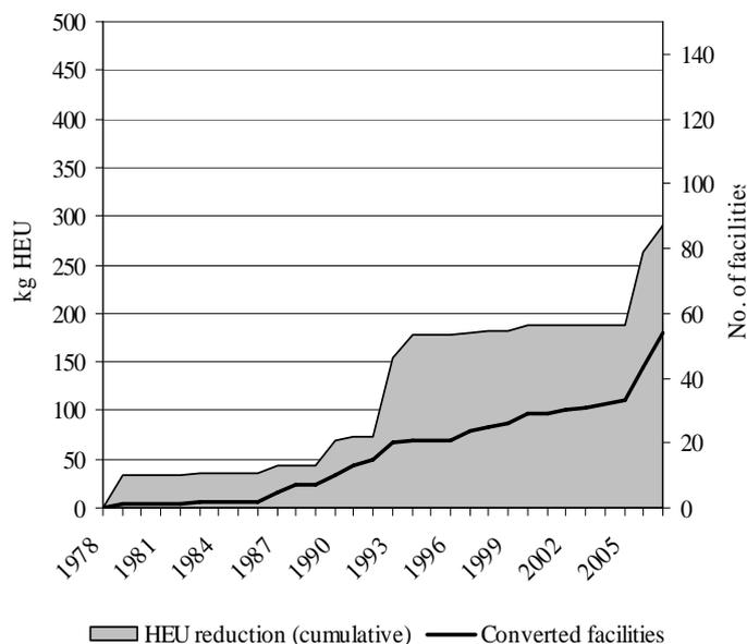
FIG. 3. Converted HEU-fueled research reactors and associated HEU consumption (kg) (cumulative) 1978–2007
