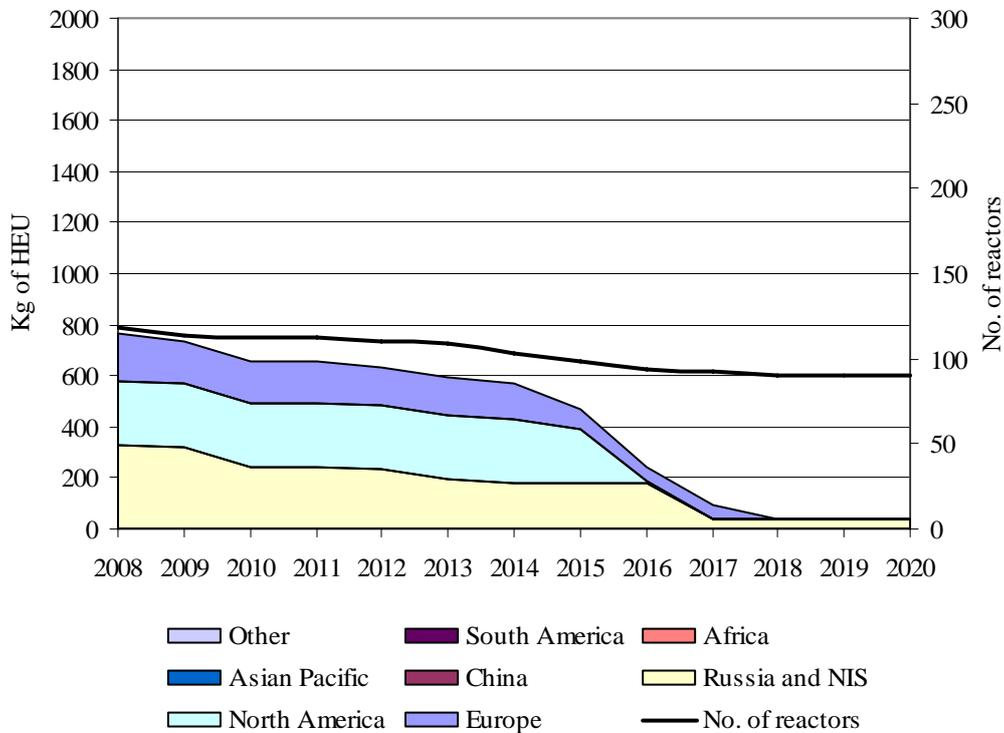
FIG. 6. Operational HEU-fueled research reactors and associated HEU consumption (kg) – Projected 2020
