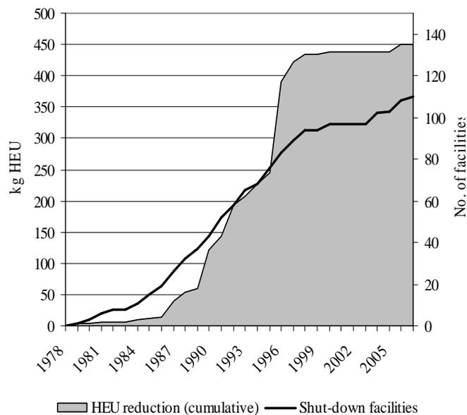
FIG. 2. Shutdown HEU-fueled research reactors and associated HEU consumption (kg) (cumulative) 1978–2007
